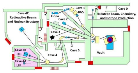
Fig. 1. Layout of the 88-Inch Cyclotron Facility.
