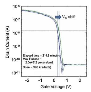
**Fig. 8.** Drain current versus gate voltage before (blue) and after (green) exposure to  $2 \times 10^{12}$  protons/cm<sup>2</sup>. The corresponding dose is 326 krads(Si). A small threshold voltage shift of less than 200 mV is observed. (For interpretation of the references to colour in this figure legend, the reader is referred to the web version of this article.)
