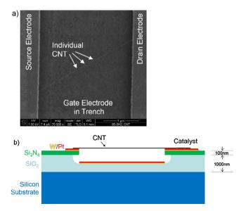
**Fig. 6.** Suspended carbon nanotube field effect transistor. (a) Scanning electron microscope image. (b) Schematic representation. Suspended portion is 500 nm to 2  $\mu$ m in length, with 500 nm of air between the gate and CNT.
