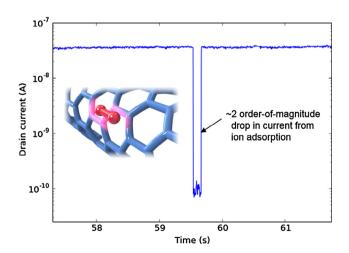
**Fig. 9.** Drain current versus time during single-gaseous ion adsorption event and subsequent desorption a fraction of a second later. Inset shows a cartoon depiction of an ionized nitrogen molecule on the surface of a CNT.
