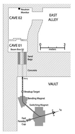
**Fig. 3.** Schematic of the thick target deuteron breakup neutron source in Cave 0 at the LBNL 88-Inch Cyclotron.
