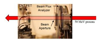
**Fig. 7.** Picture of the experimental setup. The proton beam was passed through a beam aperture and directed onto the sample in air. CNT FET devices were electrically characterized in-situ, during radiation exposure.
