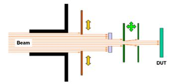
Fig. 4. Milli-Beam Schematic. The arrows show the possible motion of the different collimators.
