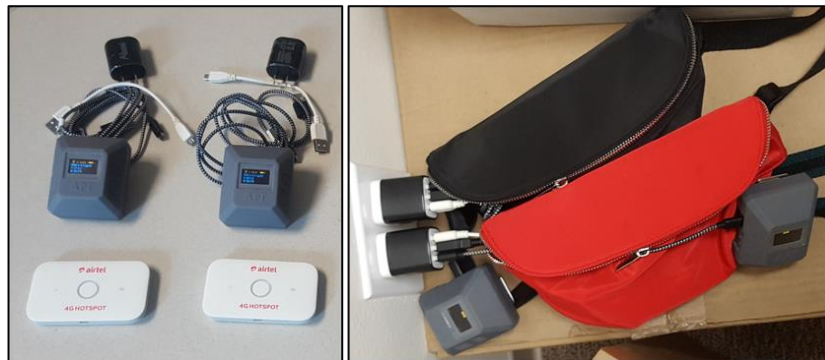
Figure 1.2. (Left) Wearable particulate matter monitors from Applied Particle Technology (St. Louis, MO). Data was transmitted via Wi-Fi hotspots and was accessible online in real-time. (Right) PM sampling pack used in the personal exposure study. The monitors were clipped outside of the pack, and the Wi-Fi and GPS data loggers were housed inside of the pack.
