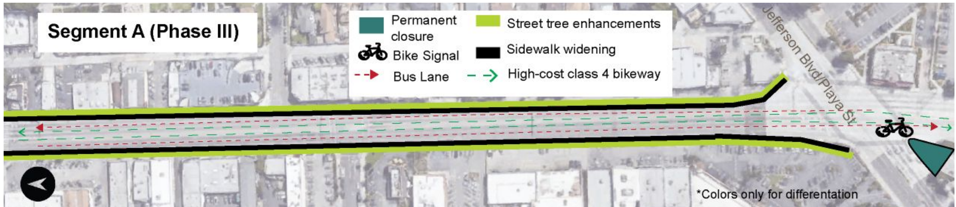
Figure 75. Segment A, Phase III recommendations
