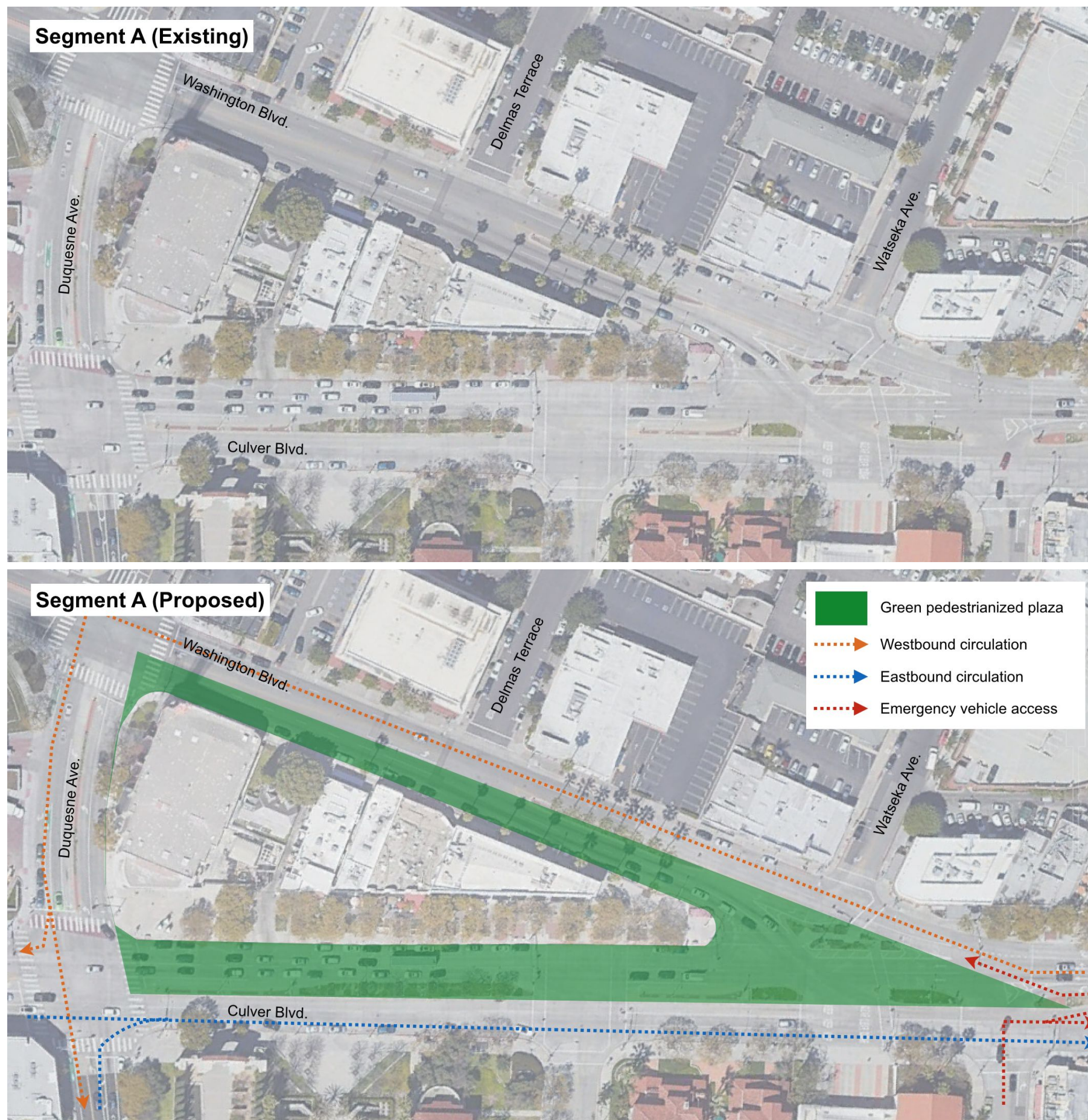
(Top) Figure 41. Existing conditions of segment A (Bottom) Figure 42. Proposed Phase III treatments for segment A
