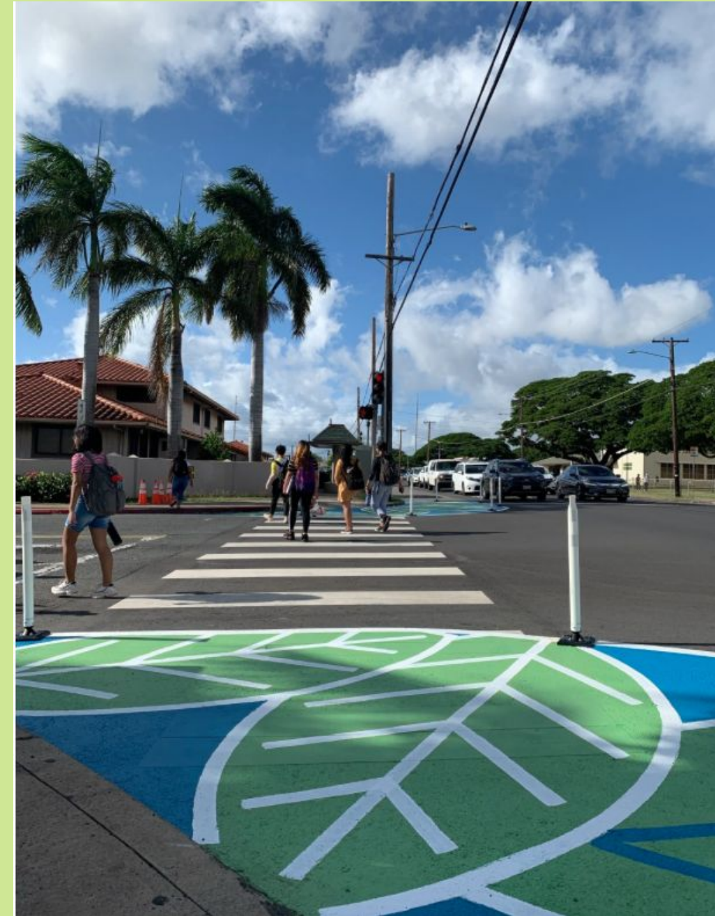
Figure 94. Tactical urbanism project for curb extension in Honolulu Source: Street Plans (n.d.)
