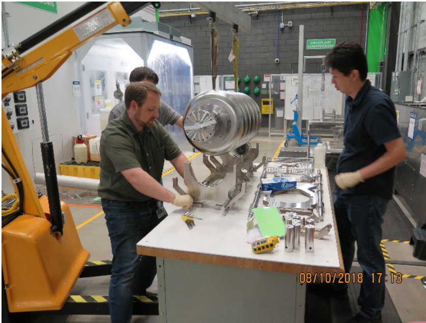
Fig. 16. SRF cavity for FRIB upgrade being processed at the MSU and Argonne National Laboratory.
