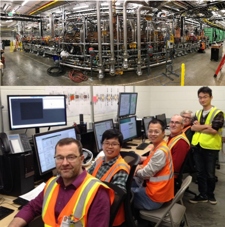
Fig. 2. Front-end (ARR1) beam commissioning in 2017. (Top) Aerial view of the room-temperature lower LEBT including the 80.5 MHz RFQ. (Bottom) Accelerator physicists and operators working at the front-end control room during the ARR1 beam commissioning.
