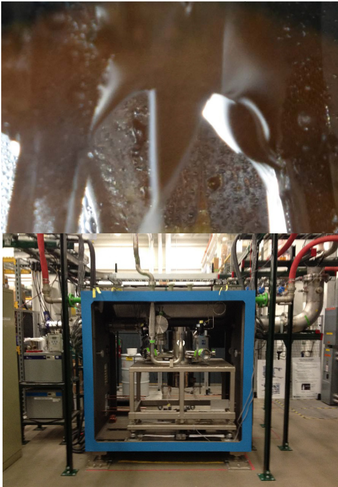
Fig. 11. Liquid lithium charge stripper module (bottom) and the established lithium film (top).
