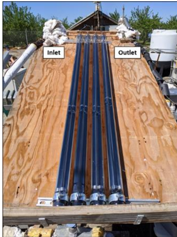
Figure 37: Integrated Compound Parabolic Concentrator (ICPC) module
