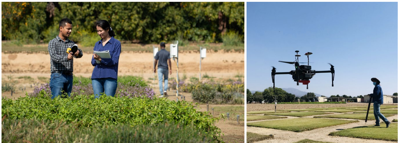
Figure 2. Students from the Verdi Water Management Group collect NDVI and canopy temperature data from groundcover species at the UCR Agricultural Experiment Station using handheld sensors (left), and from turfgrass plots at the South Coast Research and Extension Center using a drone equipped with multispectral and thermal cameras.
