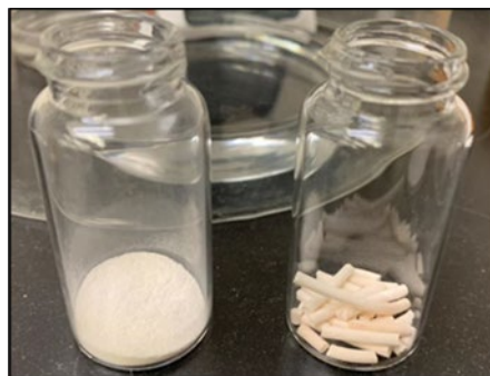
Figure 2.16. The picture of morphologies of grinded commercial NaY pellets powder and NaY pellets.
