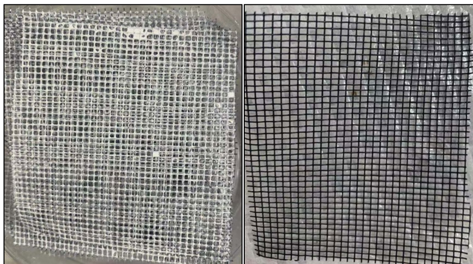
Figure 3.5. Pictures of NaY attached fiberglass(left) and bare fiberglass(right).
