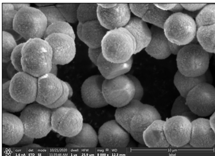
Figure 1.2. SEM image of synthesized zeolite particle using the SDA aged for 5 min under room temperature. The average size of zeolite particle is 4 \pm 0.2 \mu\text{m} .
