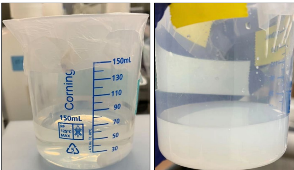
Figure S7. Photos of structure directing agent before (left) aging and after (right) 24 h aging.
