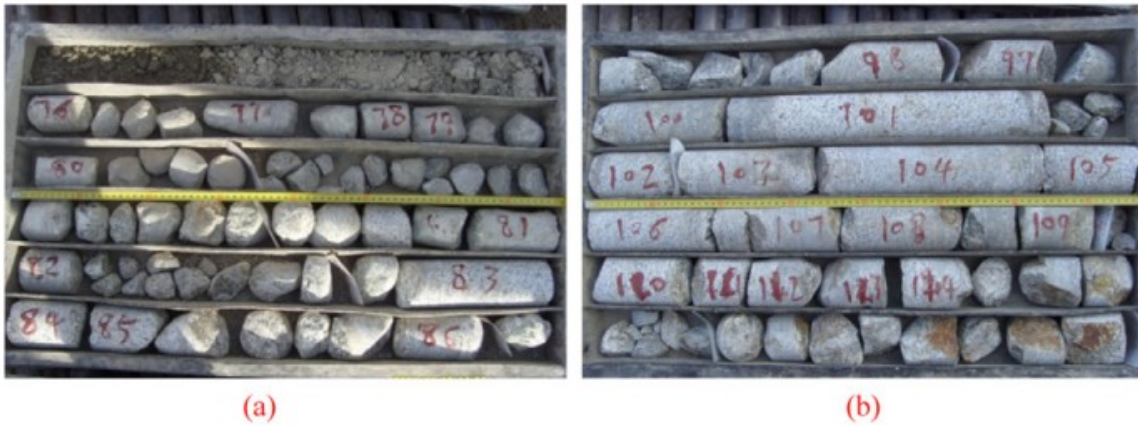
Fig. 5. The drill core of: (a) loosened fractured zone (b) heavily loosened zone.
