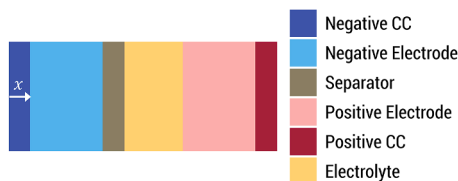
Fig. 9. Computational domain of a lead-acid battery. A flooded lead-acid battery has all the indicted domains, but a VRLA does not have an electrolyte reservoir because the electrolyte is immobilized in the separator.
