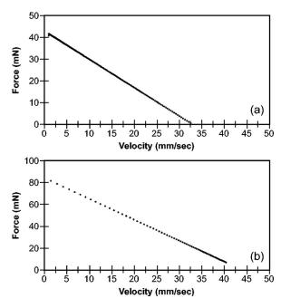
0.45 N preload on the contact interface. Using a single point FIG. 4. Sliding force vs velocity: (a) leftward and (b) rightward. Downloaded 22 Jan 2008 to 130.194.10.86. Redistribution subject to AIP license or copyright; see http://apl.aip.org/apl/copyright.jsp
