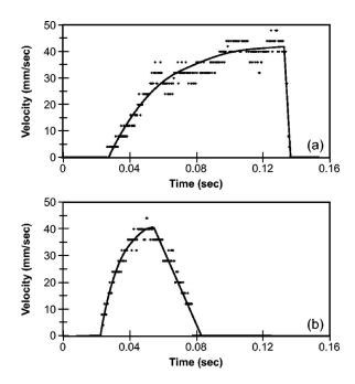
FIG. 3. Velocity vs time for a single run: (a) leftward, 1.733 MHz, and (b) rightward, 1.823 MHz.
