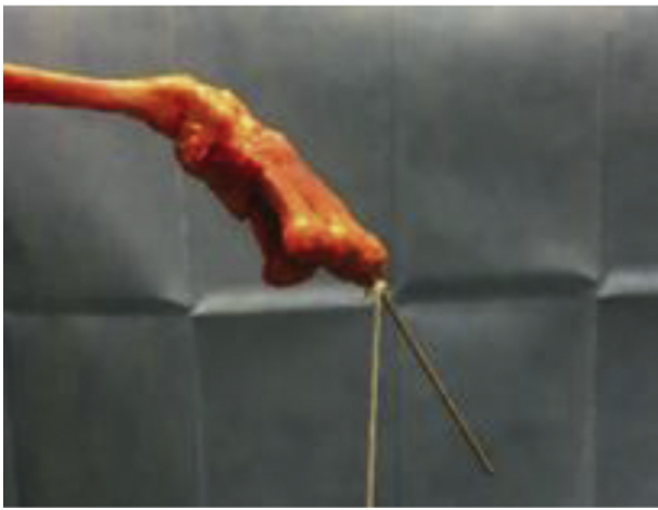
FIGURE 1: Image depicting the technique for simulating wrist flexion using a traction weight applied to the third metacarpal.
