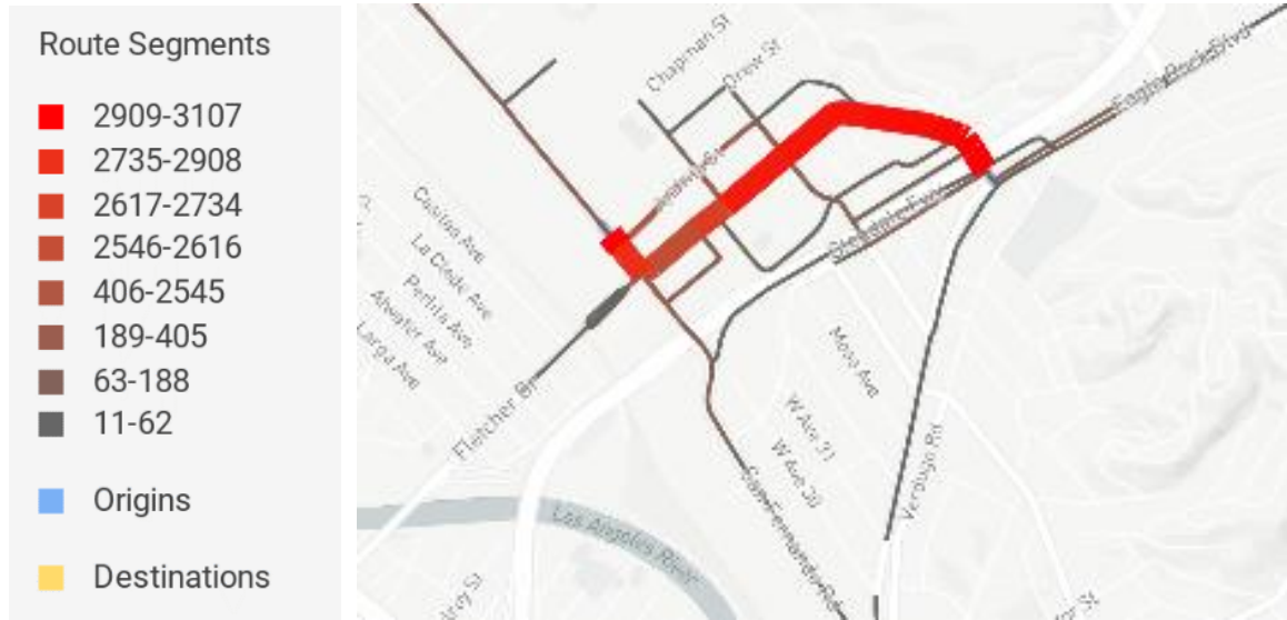
Figure 13. Fletcher 2019 Cut-Through Map: A small increase in cut-through traffic is observed on Fletcher Drive after the road diet implementation.
