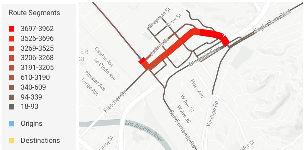
Figure 13. Fletcher 2019 Cut-Through Map: A small increase in cut-through traffic is observed on Fletcher Drive after the road diet implementation.
