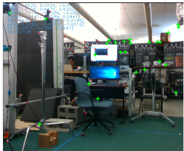
Figure 2.2: Example Module Outputs. Left: An example output image of our trained object detector using a custom-trained convolutional neural network model. We used the YOLOv3 [RF18] architecture with default initialized weights for fast training and inference. Right: Inlier (green +) and outlier tracks (red *) produced by XIVO on data collected from the Intel Realsense D435i.
