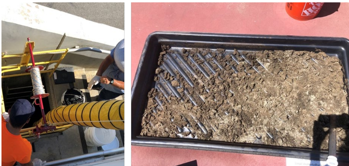
Figure 5-1. (left) Collection of the drinking water treatment residuals in the Groundwater treatment plant in Long Beach. (right) drying process of the drinking water treatment residuals on the roof in August 2022.
