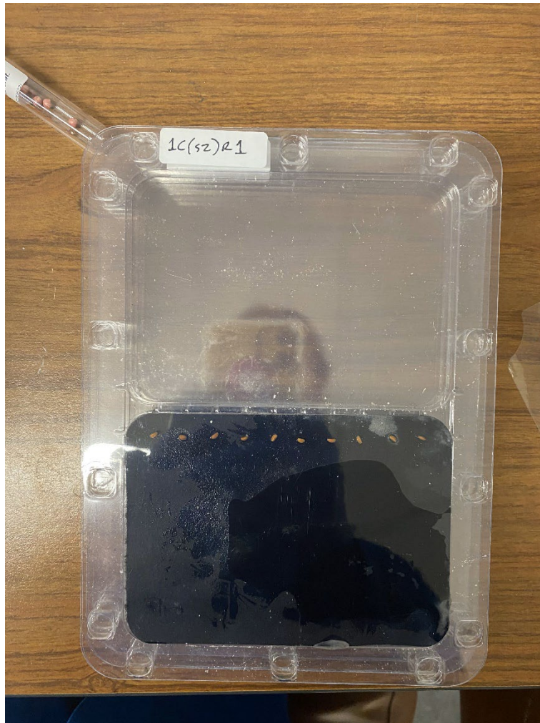
Figure 4-2. A test plate before the incubator with the 10 seeds and the black filter on top of the soil.
