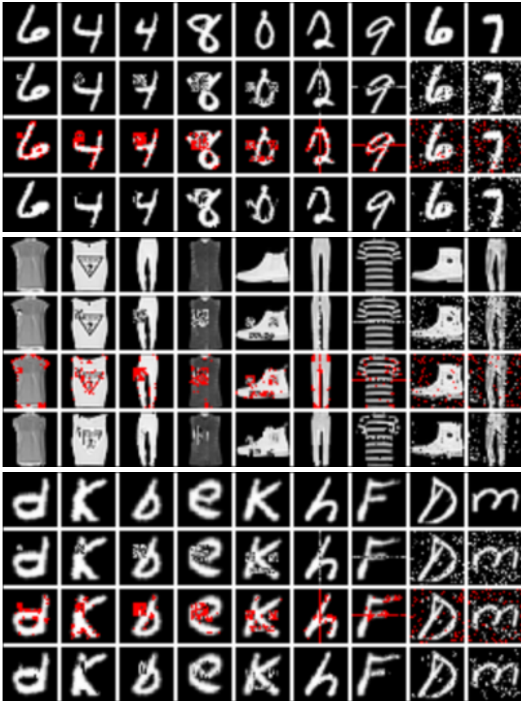
Figure 6.1: Effective outlier feature detection with inlier maximization with a fixed budget. Each row corresponds to (top to bottom): original images, corrupted images, outliers found with budget k = 60 (denoted with red pixels), and images that have been cleaned by the generative model. Each column corresponds to a different corruption process (left to right): Square(3x3), Square(5x5), Square(7x7), Square(9x9), Smiley, Column(14), Row(14), Random(120), Random(200).
