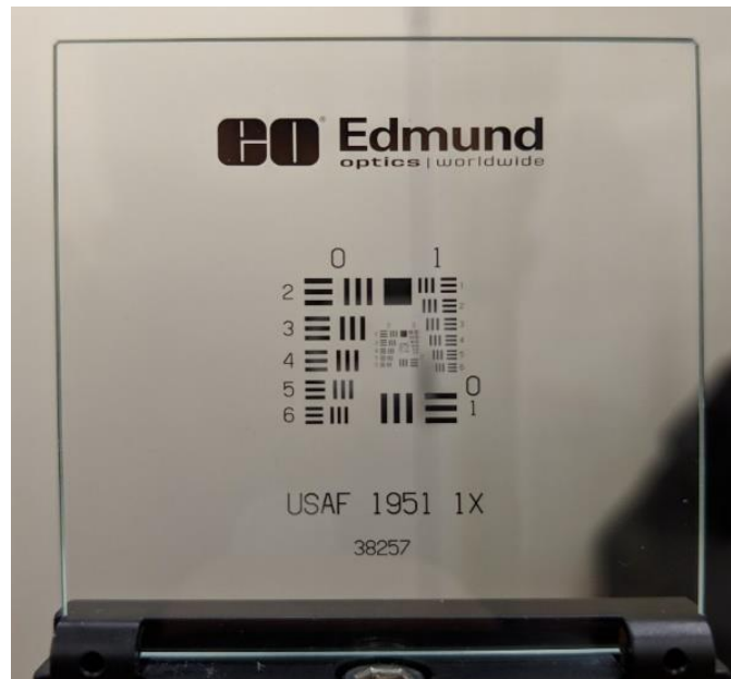
Figure 5 A USAF 1951 air force target used to determine the lateral resolution of the spectroscopic OCT system.
