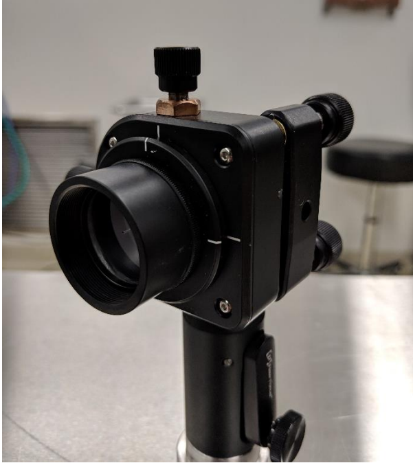
Figure 7 The phase plate mounted into a 5-axis kinematic mount. The 0.5mm diameter hole at the center of the phase plate will create a difference in the optical path length and help improve spectroscopic resolution. The micrometers will assist in properly aligning this optical component at the center of the beam path.
