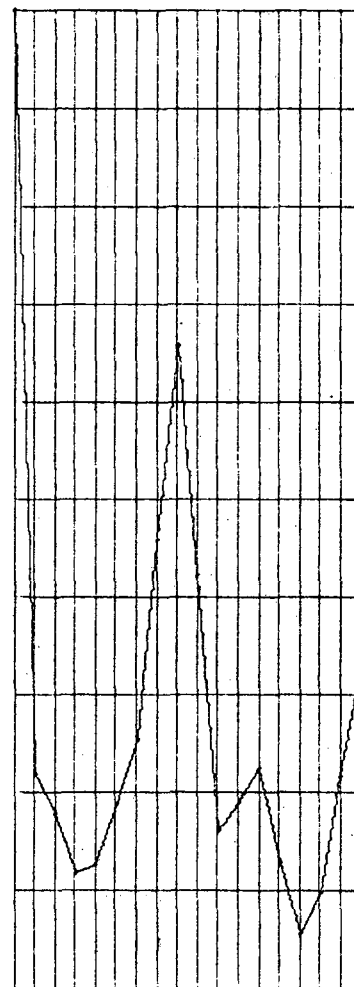
Fig. IV-6a. I_{00} vs eV for Al (100) between 19 and 36 eV at \theta = 0^\circ calculated with \lambda = 1.0\text{\AA}^{-1} , \alpha = 0.9 , T = 300^\circ\text{K} , \theta_B = 400^\circ\text{K} , \theta_S = 200^\circ\text{K} for several values of the parameter \nu . Fifteen scattering events were employed and the four beam approximation was made.
