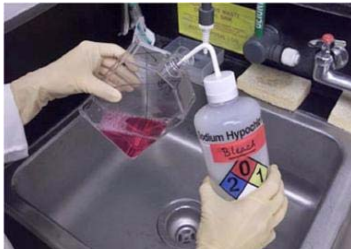
Figure 2-9. To disinfect your liquid waste, create a 10% concentration of household bleach in the liquid waste.
