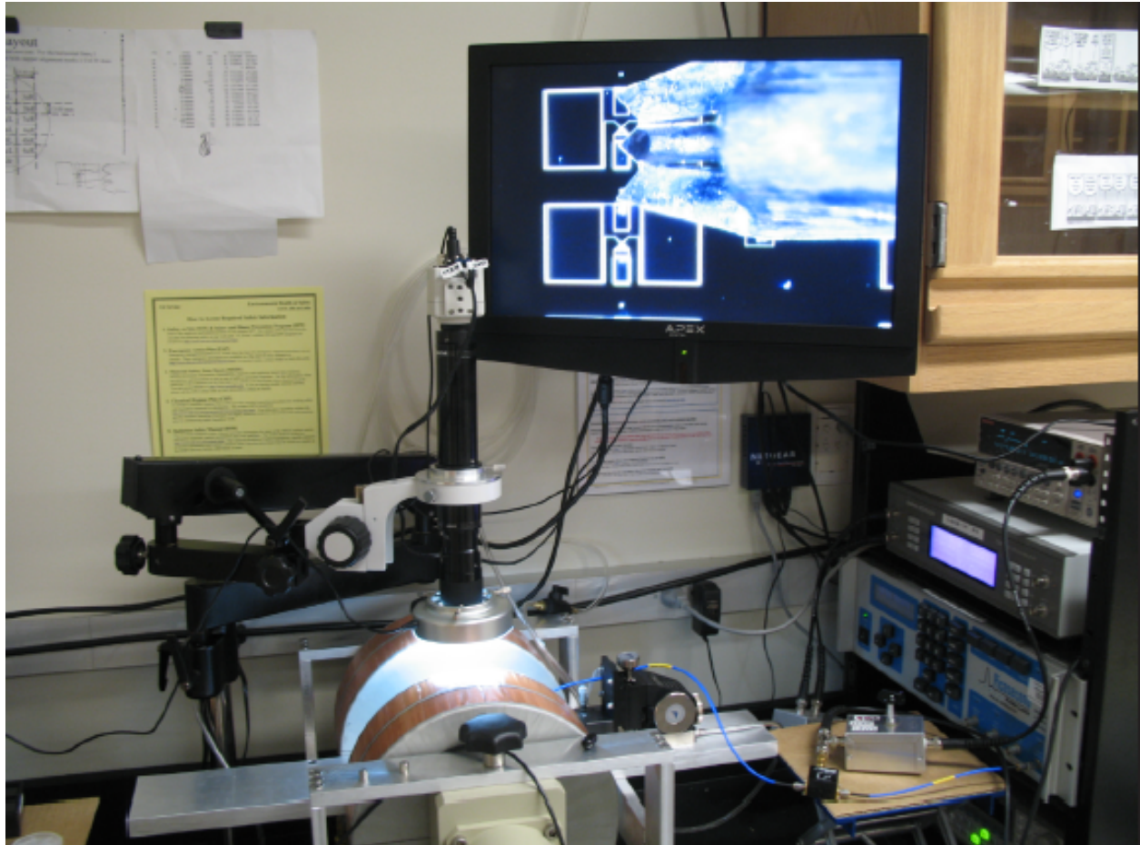
Figure 2.1: [1]Photograph of the probe station. The optics, ring light and a monitor are hooked up to the CCD to project and enlarge the sample image. A 200\ \mu\text{m} pitch microwave probe is positioned to touch down onto a typical sample's leads.
