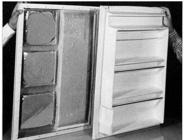
Gas-filled panels: An effective new CFC-free insulator for refrigerators and many other applications.
