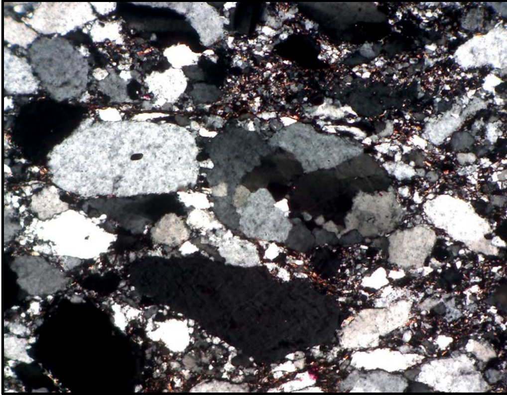
Figure 19. Photomicrograph (x-nicols) of typical Shoo Fly sandstone showing sub-angular to sub-rounded quartz framework grains oriented parallel and sub-parallel to foliation. The image also shows the apparent bi-modal size distribution that is common to the Shoo Fly sandstones and the mix of monocrystalline and polycrystalline grains.
