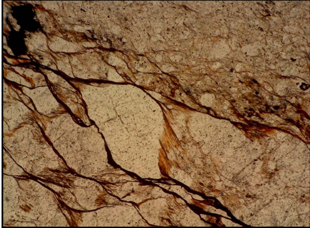
Figure 22. Same image as 21, but in plane-polarized light. The image also shows the development of “beards” or “trains” of matrix phyllosilicates and quartz in pressure shadows at the ends of and between quartz grains in response to deformation-induced pressure solution (DeVay, 1981).
