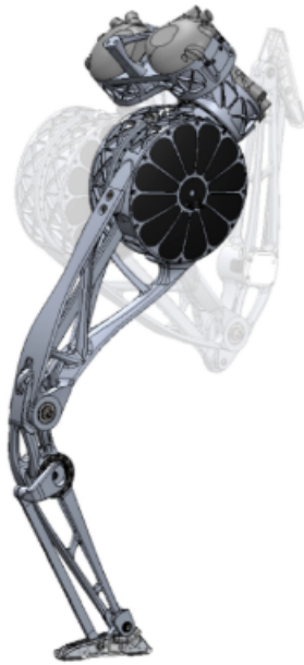
Figure 3.5: Since Artemis only has a 5 DoF leg (no ankle roll), the platform behaves very similarly to the LIP model in real life due to the lower distal leg inertia and the ankle naturally rolling about the contact point
