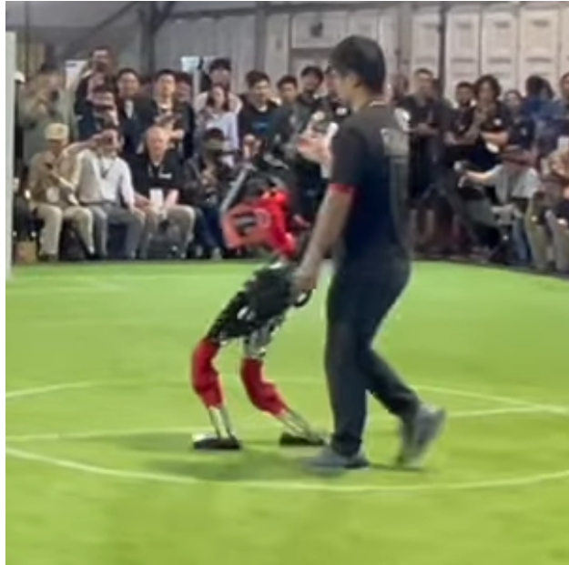
Figure 5.2: During longer strides, Artemis become kinematically limited. To reach faster speeds, either shorter timings, non parallel foot landing sequences, or running must be performed.
