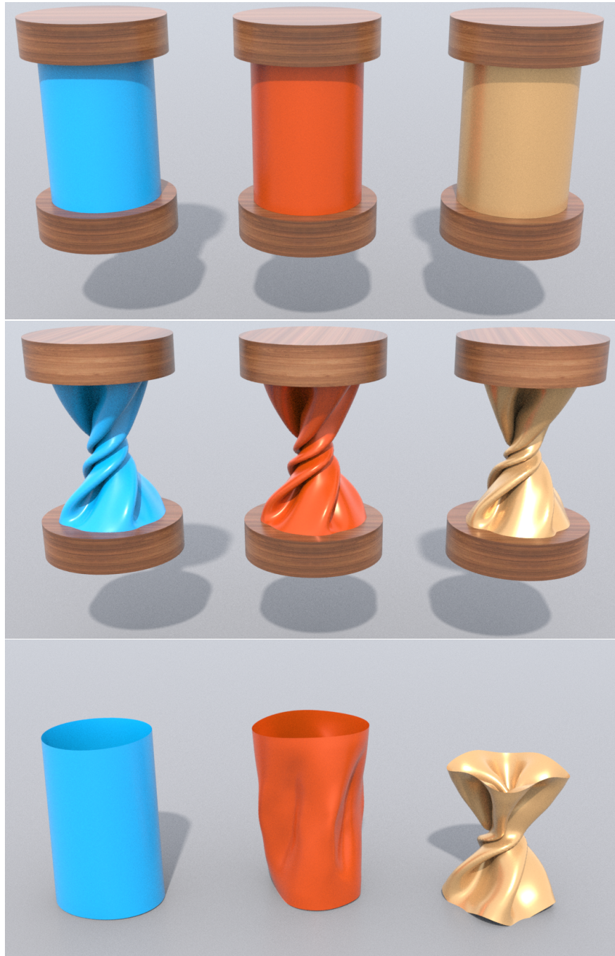
Figure 5.14: Plastic shell deformation. The effect of the yield condition in Equation (5.13) is shown here with decreasing values of the coefficient c_{vM} (from left to right). Larger values correspond to a larger stress needed for before denting plasticity is induced. The cylinders are twisted and then dropped to the ground to illustrate the plastic deformation.
