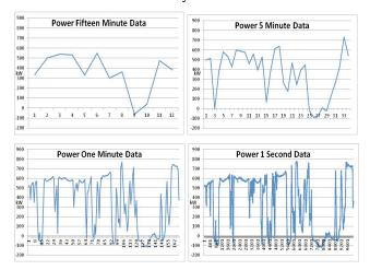
Output variation from a PV array, as observed at different time resolutions, illustrates the need to look more closely at distribution systems: depending on the granularity of the measurement, the data tell a different story.
