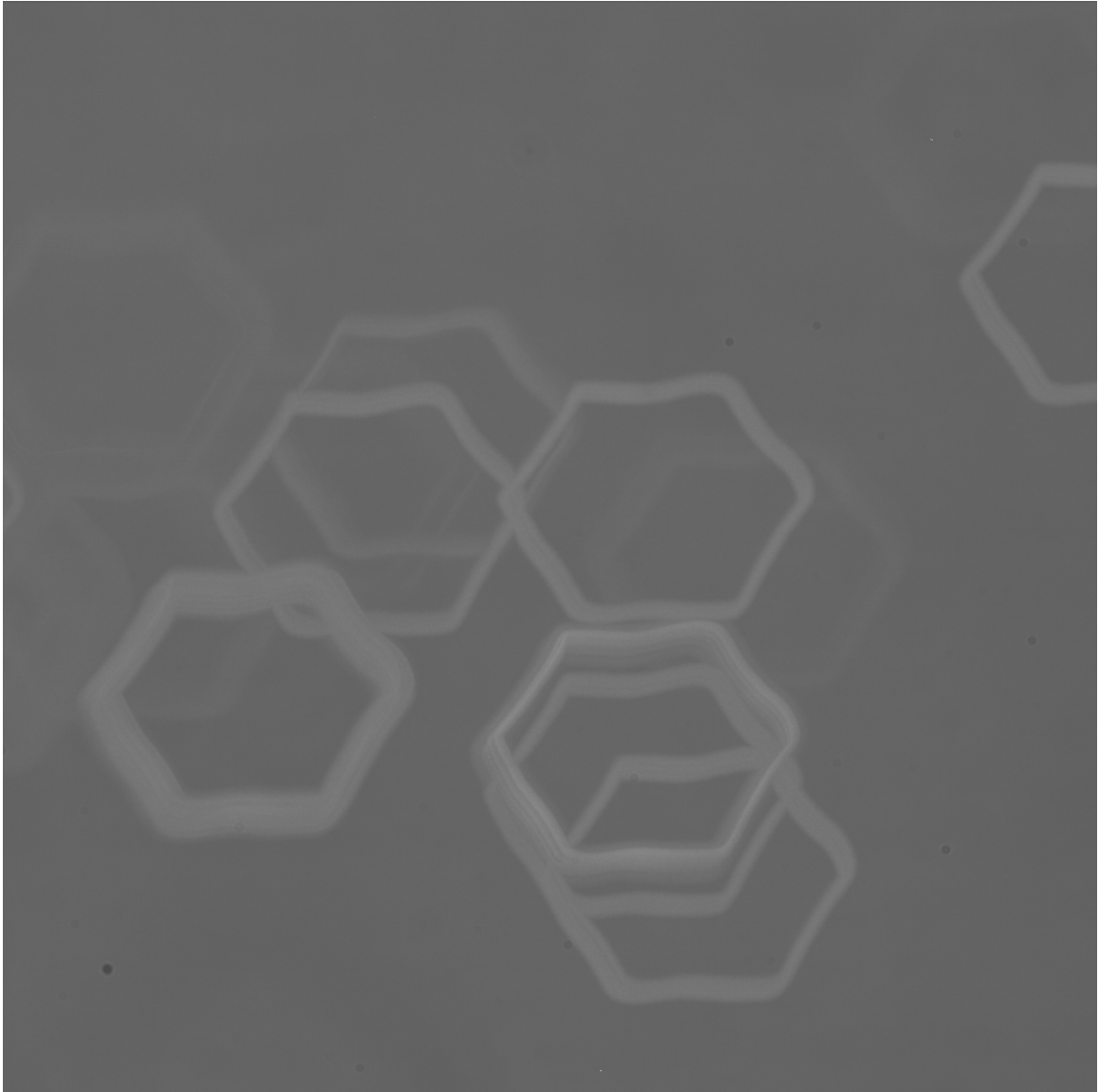
Figure 4.4: Time lapse image of 2 \mu\text{m} latex tracer particles moved inside microfluidic manipulator tracing out a hexagon with constant angular velocity. Window size is 188 \mu\text{m} \times 188 \mu\text{m} .
