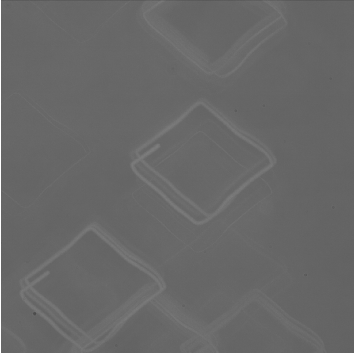
Figure 4.3: Time lapse image of 2 \mu\text{m} latex tracer particles moved inside microfluidic manipulator tracing out a square with constant angular velocity. Window size is 188 \mu\text{m} \times 188 \mu\text{m} .
