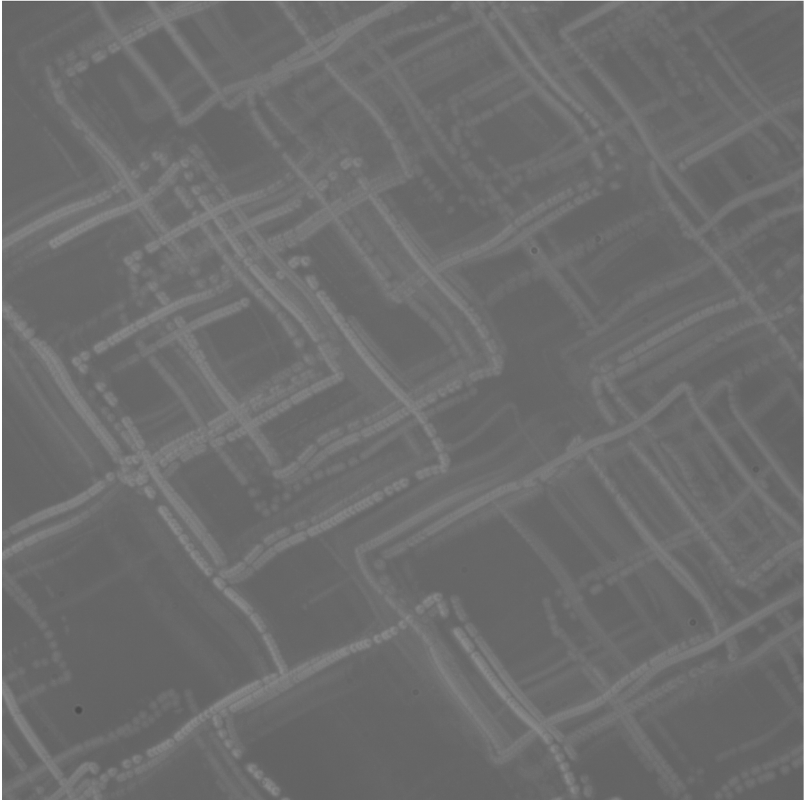
Figure 4.7: Time lapse image of 2 \mu\text{m} latex tracer particles moved inside microfluidic manipulator tracing out an experimentally integrated square via conformal mapping. Window size is 188 \mu\text{m} \times 188 \mu\text{m} .
