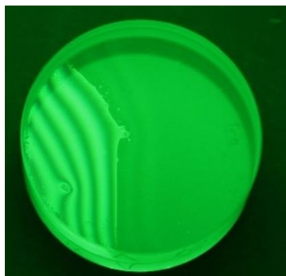
Figure 18. Fused silica sample displaying a bond-front with trapped particles. The transparent region represents well-contacted areas. The cloudy region displays interference fringes that suggest non-contacted areas.
