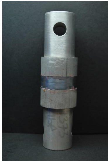
Figure 19. A silicon sample epoxy-bonded to custom aluminum fixtures made in-house for flatwise tension experiments.
