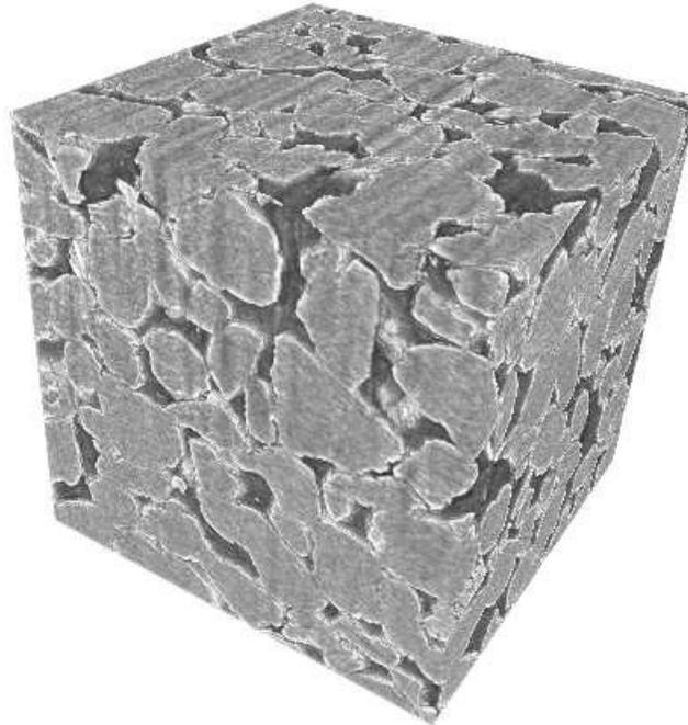
Figure 4. Gray-scale 750×750×750 voxels image of Bentheimer sandstone obtained at the Advanced Light Source Facility at LBNL. Voxel size is 4.42 micron.
