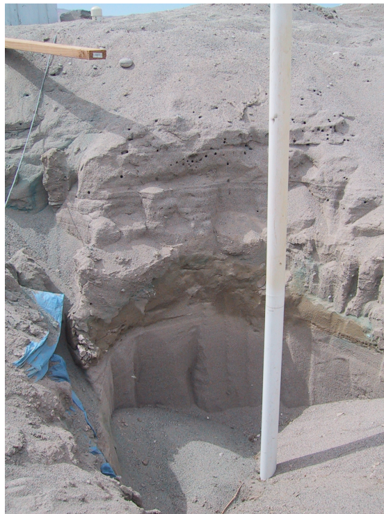
Figure 22: Photograph of visibly wet sill north of the drip line and west of the dike.
