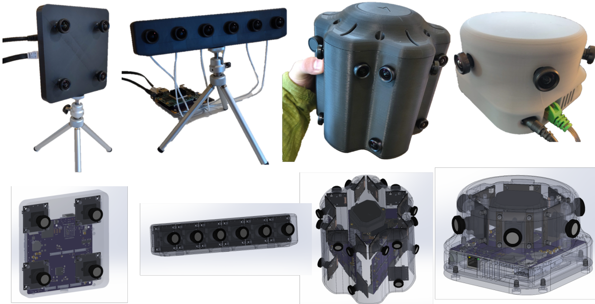
Figure 6.11: DevCAM Mechanical Configuration Variants- from left to right: Quadnocular, Co-linear Lightfield, Trinocular Panoramic, Panoramic
