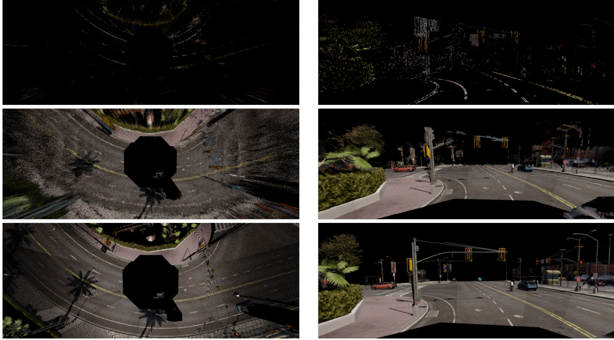
Figure 7.9: Synthetic Reconstruction Evaluation in Bird's Eye View and Side-view: (top) Semi-dense contour reconstruction, (middle) Dense Semi-Global Matching, (bottom) Ground Truth.
