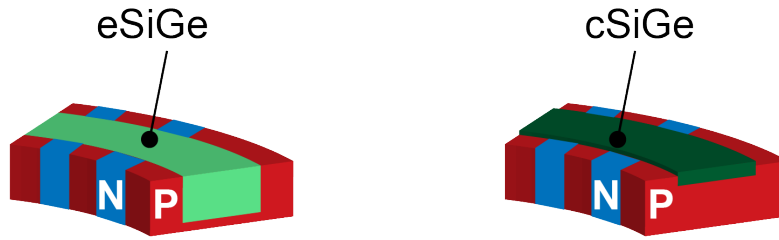
Figure 4.12: Cross-section of eSiGe- and cSiGe-based resonant PDs in the zero-change 32 nm platform.
