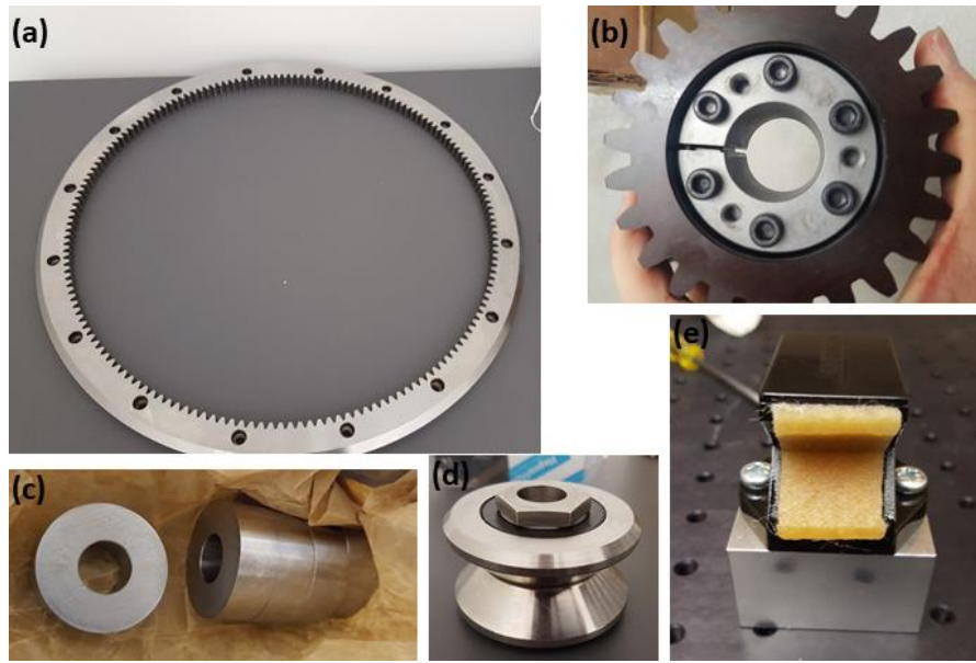
Figure 5.19. Heavy-duty ring track for FXLT imaging system. (a) Ring track; (b) Pinion; (c) spacers; (d) bearings; (e) lubricators.
