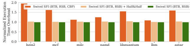
Figure 12: Performance overhead of Half&Half (Swivel) on SPEC 2006 benchmarks.
