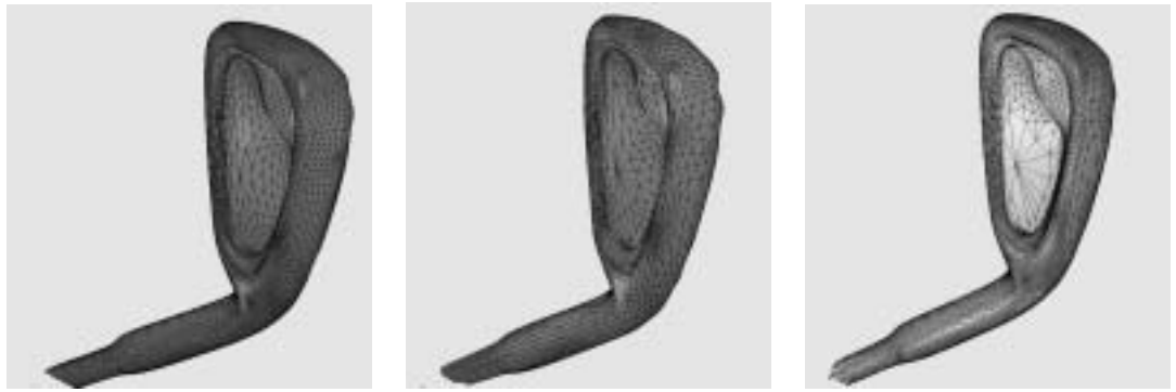
Figure 5: Comparison of normal subdivision, dihedral angle adaptive subdivision and watershed adaptive subdivision applied on to a golf head file
