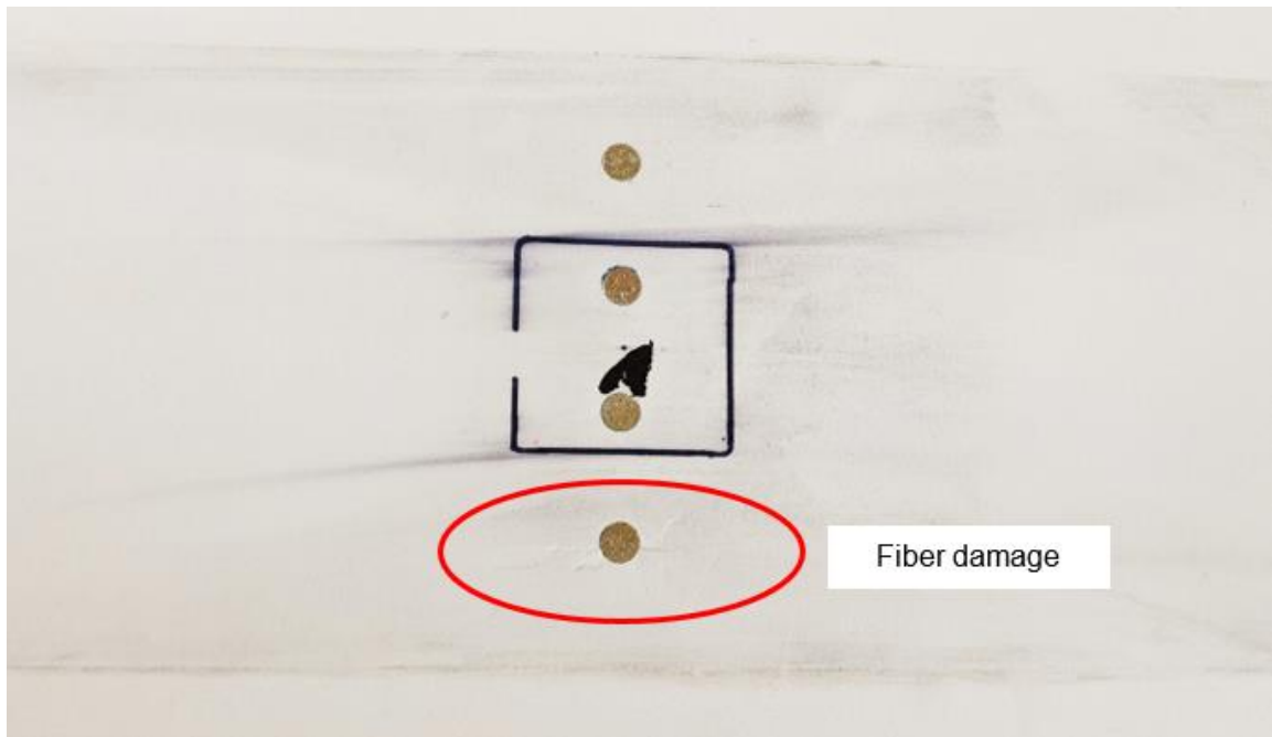
Figure 3.101: Barely visible skin crack at skin bolt after Loc3-2 test.
