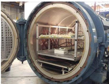
Figure 3.22: 1.8 m diameter autoclave in San Diego Composites (left) and autoclave cure cycle (right) [26].
