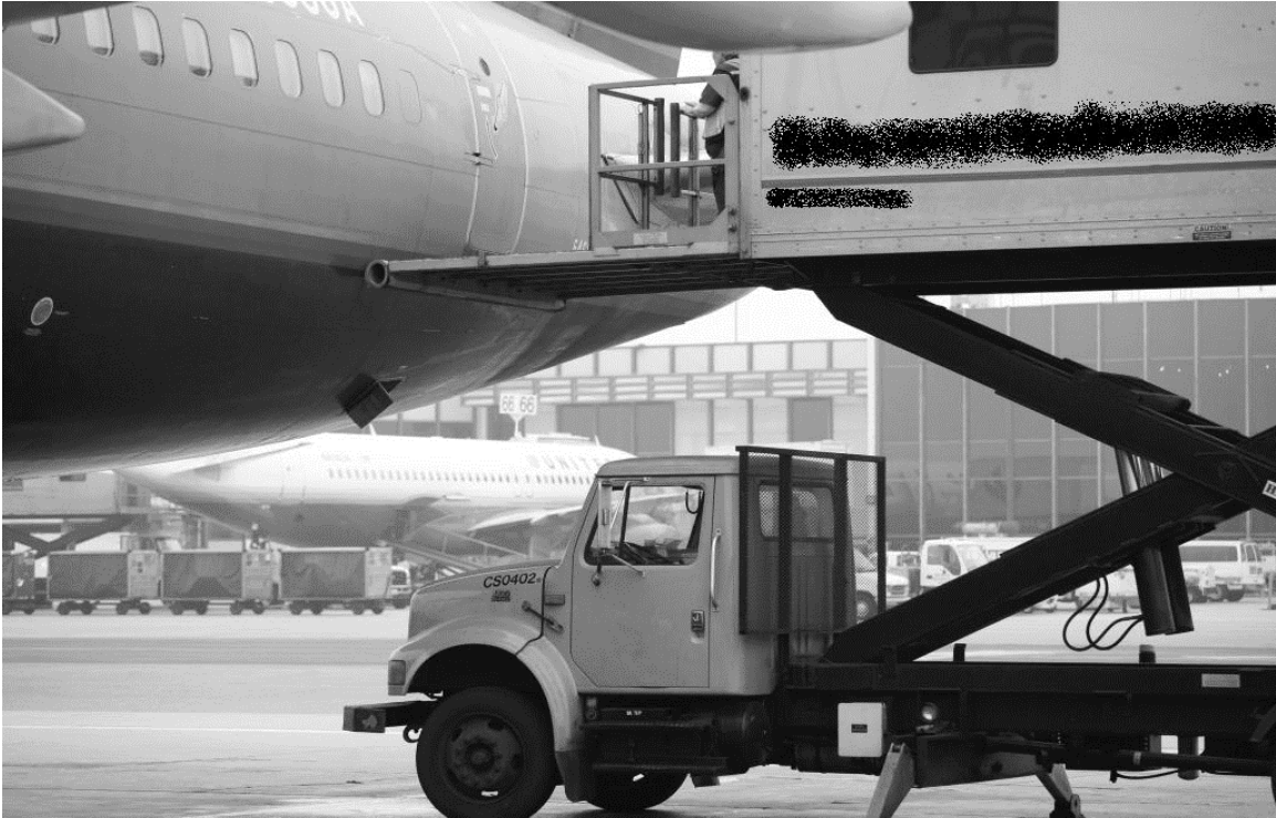
Figure 1.3: GSE approaching to the aircraft fuselage; note rubber bumper at interface between GSE and aircraft [8].
