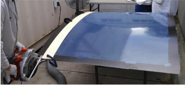
Trimming the co-cured skin-stringer part
