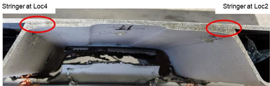
Figure 3.81: Visible skin-stringer disbond after Loc3-2 test.
