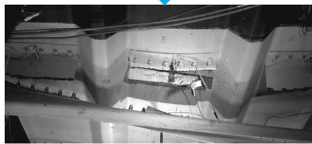
Figure 2.5: Internal damage sequence of Frame03 panel loaded onto shear ties [8, 11].
