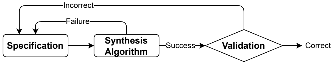
Figure 1.1. The stages of synchronous program synthesis. Respecifying and repairing incorrect solutions may be considered separate stages, but here they are folded into “Specification” and “Validation” respectively.
