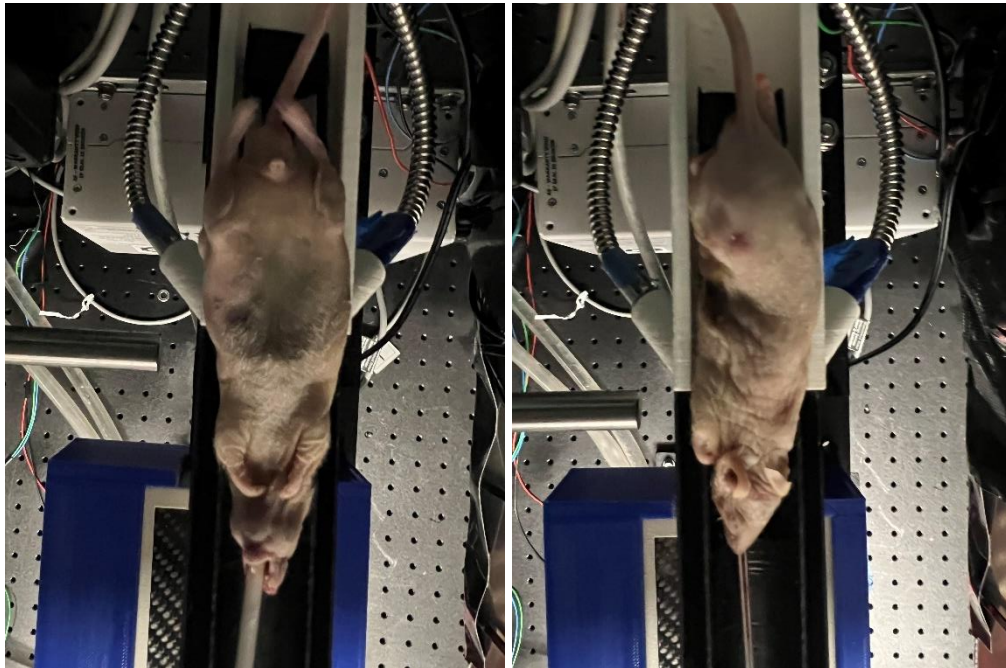
Figure 5.2. The euthanized mouse embedded with one capillary tube target (left) and the euthanized mouse embedded with three smaller capillary tube targets (right).
