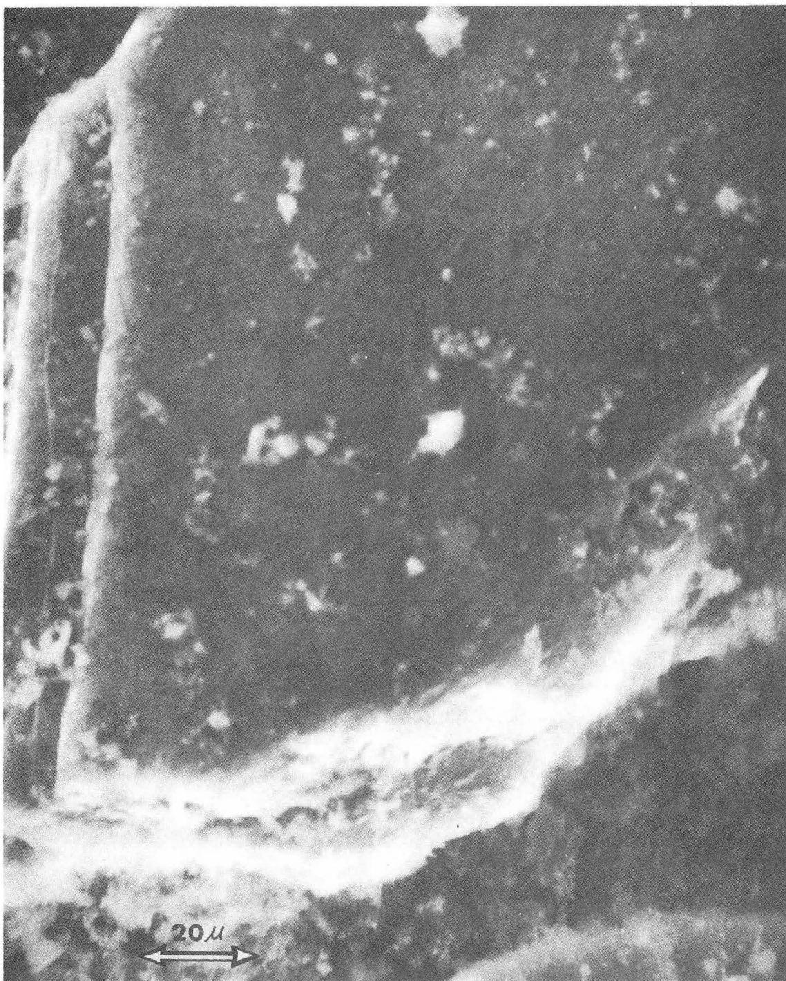
Fig. 37 Scanning electron micrograph of magnesium nitride particle from material prepared in this laboratory.
