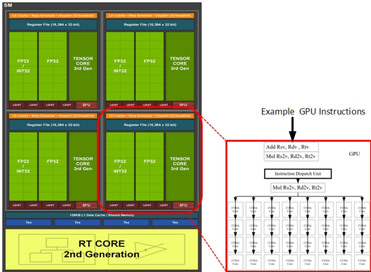
Figure 2.6: Architecture of a Streaming Multiprocessor (SM) unit inside Nvidia GPU [36], and an example warp dispatch.
