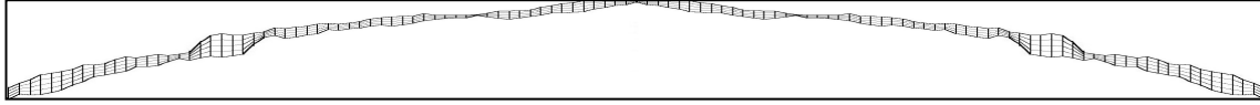
Figure 2. An example of fracture models showing various roughness and apertures at each stage. Exaggerated 50 times in vertical direction.
