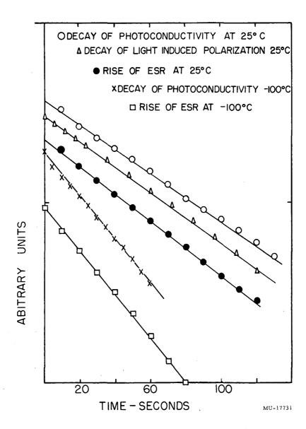
Fig. 3. Semilog plots of time dependence of photoconductivity, light-induced ESR, and light-induced polarization in doped phthalocyanine. The relative positions of each of the curves in this figure are not comparable.
