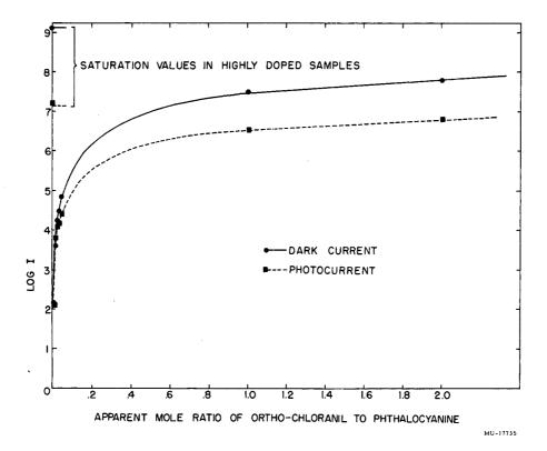
Fig. 1. Variation of dark conductivity and photoconductivity of phthalocyanine with amount of ortho-chloranil added.
