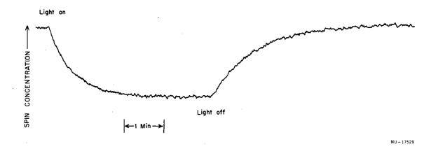
Fig. 5. Effect of illumination with white light on the ESR signal in ortho-chloranil-doped phthalocyanine. Curve represents unpaired spin concentration vs time.
