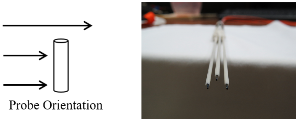
Figure 3.6: Langmuir probe configuration for the 1D (a) and 2D (b) [2] experiments.
