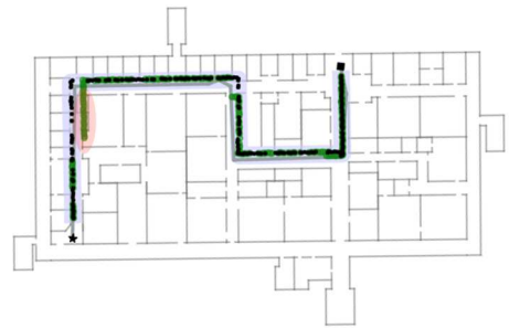
Fig. 8. See caption of Fig. 6. Comparison of return paths using hybrid matching with different LRP definitions. Black lines represent paths using hybrid matching with machine learning ( LRP_{NN} , determined by FCN). The green line is the path using hybrid matching with a linearly defined LRP ( LRP_{local} ).
