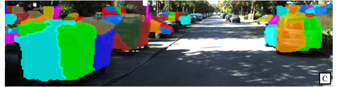
Fig. 7: A sample scene from KITTI containing obstacles of different classes, with (a) LiDAR measurements and (b) image data. Super-surface segments are extracted for non-ground points in (c).
