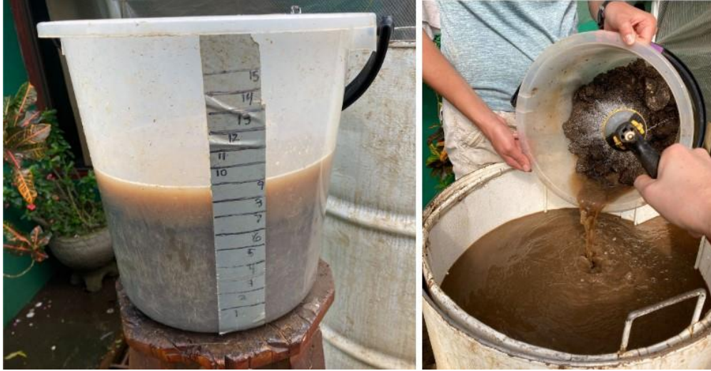
Figure 6-28: Left: Measurement of soil samples using water displacement. Right: The bucket used for measurement of the sample is slowly poured into the main tank with the aid of a water hose.
