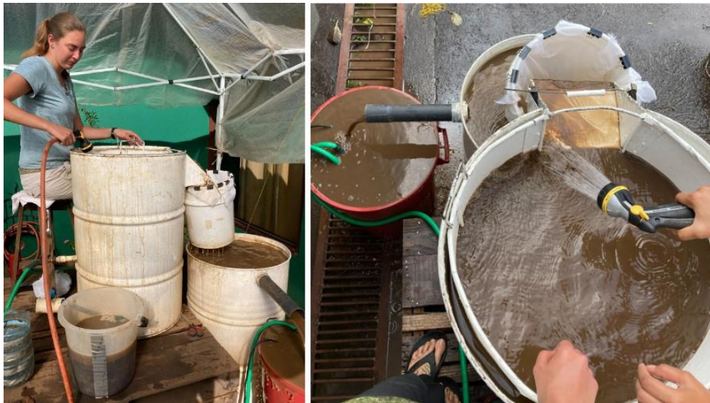
Figure 6-27: Images showing the flotation tank system in operation, which made use of a series of settling tanks to recycle water.
