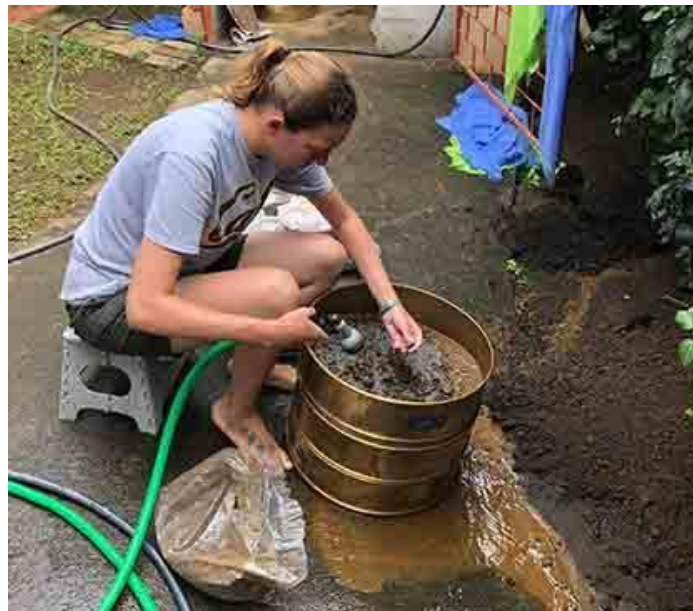
Figure 6-10: Author processing water screened samples using a series of geological sieves (4mm, 2mm, 0.5mm).
