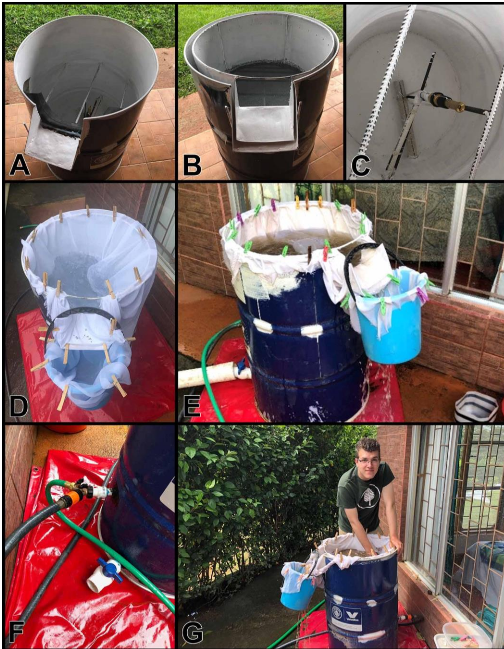
Figure 6-7: The flotation tank system at La Chiripa: A) The main tank showing the placement of the support rods for the inner basket and the rubber tire sealing the light fraction exit and preventing water from exiting the tank below the heavy fraction basket. B) The main tank with the heavy fraction basket inserted in place. C) Interior of main tank with a view of the water spout with its support rod and the exit pipe below to empty the tank's contents. D) The flotation tank with heavy fraction mesh and light fraction mesh held in place using clothespins. E) View of the flotation tank when a sample is being processed within. F) View of the entrance and exit piping configuration. The entrance uses a splitter so that some water can also enter a small hose to spray the sample contents during processing. G) View of the flotation tank while being operated by project member Andrés Mejía-Ramón. The system was donated to the Museo Nacional de Costa Rica at the end of the field season.
