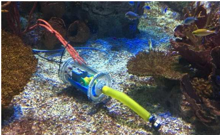
Figure 13: The eversion robot was tested in a coral reef tank at Birch Aquarium in SIO. (a) A diver assisted in the deployment of the robot to collect data of coral reef structures. (b) The base chamber of the body remains stationary, while the soft fabric body is able to grow through the passageways of coral reefs with the goal of acquiring transects to translate the structures into 3D models for studying the health and ecology of various species.
