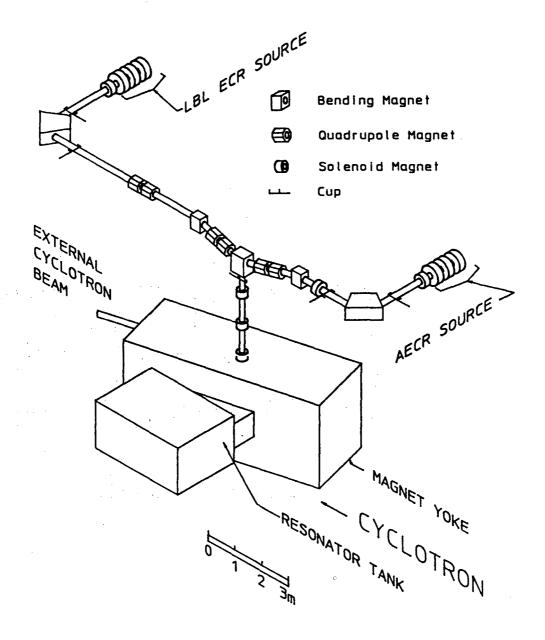
Fig. 1. Schematic view of the injection beam transport lines for the 88-Inch Cyclotron, from the LBL ECR and the AECR sources. Either of these two ion sources can inject beams into the cyclotron. XBL 915-1071.
