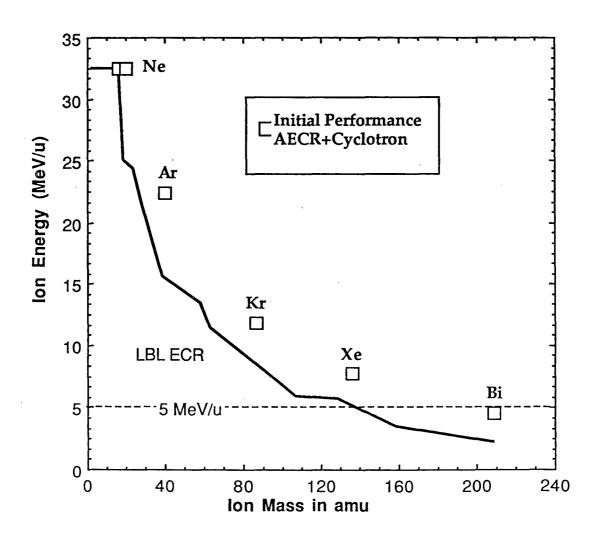
Fig. 3. The best performance of beams accelerated by the LBL ECR and the AECR sources in the 88-Inch Cyclotron. XBL 915-1073.
