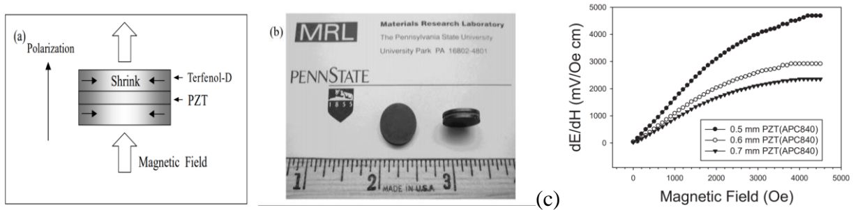
Figure 1.6. Magnetoelectric lamina composite using TERFENOL-D and PZT disks. (a) schematic structure, and (b) photograph of the device. (c) Magnetoelectric voltage coefficient as a function of applied d.c. magnetic bias with various thickness of PZT layer at 1 kHz [18].
