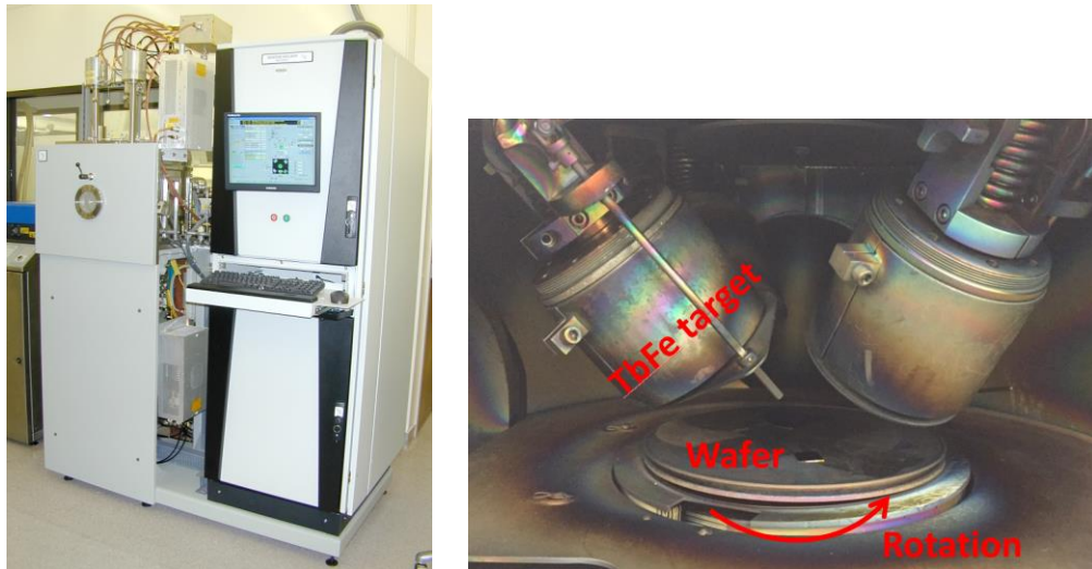
Figure 3.12. Denton sputter deposition tool. (Left) Exterior of the tool installed in the class 1000 HEPA filtered cleanroom facility (Right) Inside of the vacuum chamber showing the angled sputtering guns and rotating substrate holder.
