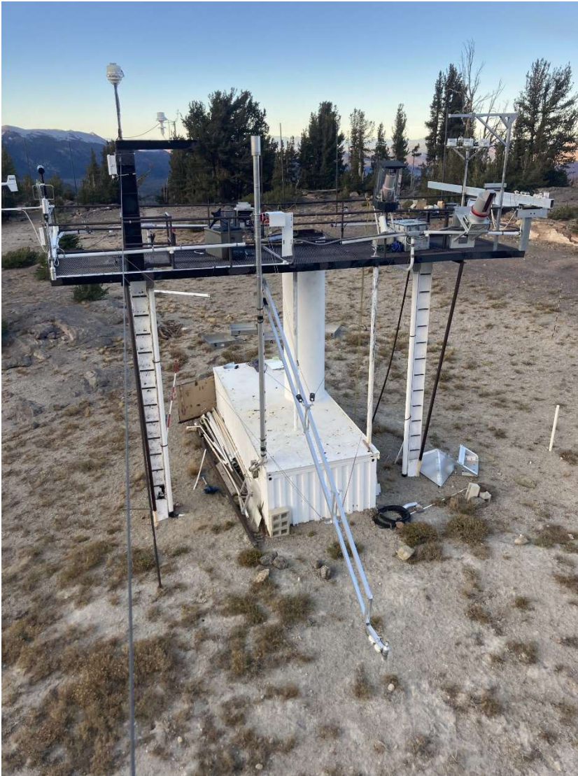
Figure 3: The CUES platform in 2020 with its wide array of instruments. The movable arm is seen in the foreground. https://snow.ucsb.edu/index.php/2020/09/23/2020-cues-tlc/
